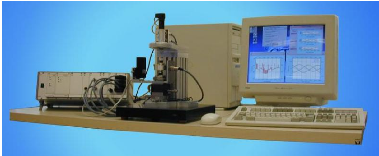
FIGURE 1: Micro torque testing stage with electronic rack (left), mechanical setup (middle) and computer.
