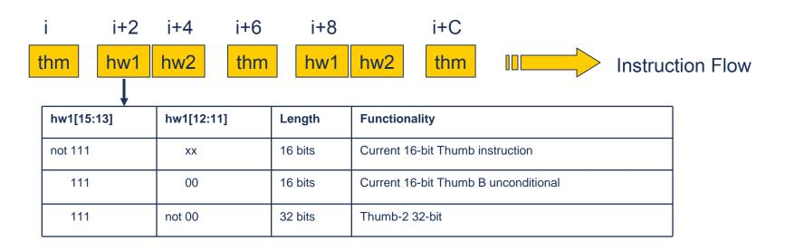
Halfword pairs (hw1, hw2) of instructions are inserted into Thumb (thm) instruction stream.
