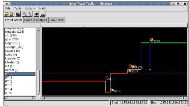
FIGURE 4: A safe environment (RT1) to destroy real time tasks - LTT capture
