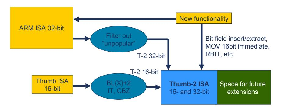
The ARM Thumb-2 core technology combines 16- and 32-bit instructions in a single instruction set and allows programmers / compilers to freely mix the instructions together without mode switching.
