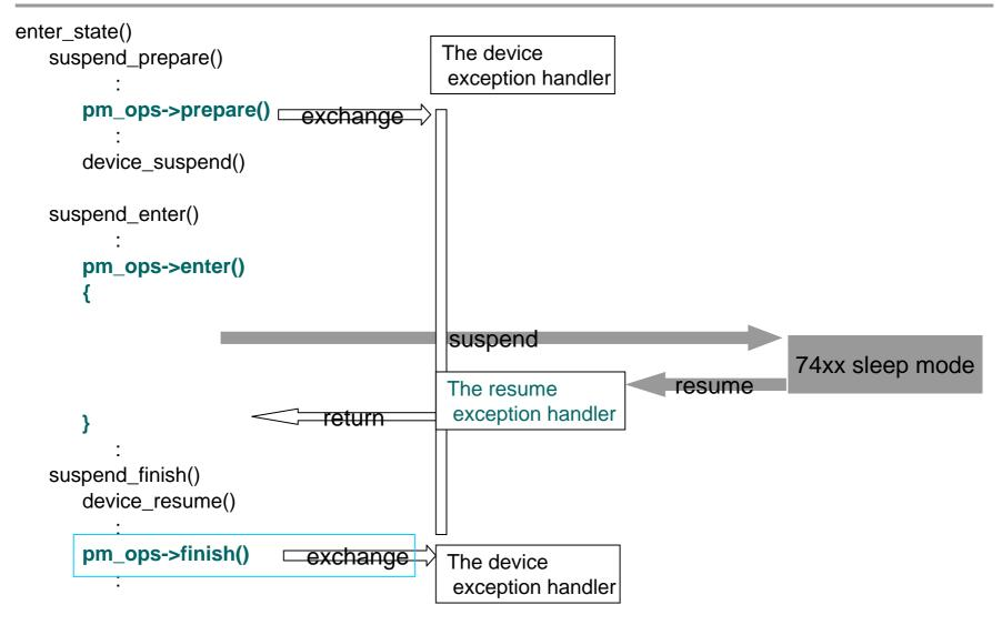
The postprocessing dependent on the CPU architecture is wrapped in pm\_ops ->prepare() function.
