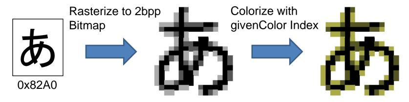
■ To realize this process, 2bpp pixel format and CLUT conversions are added.
