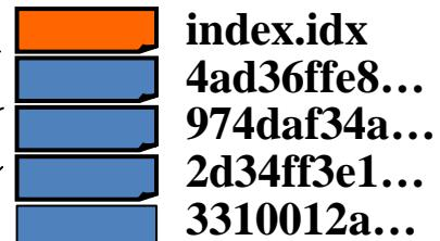
The block files are reconstructed as a virtual disk with HTTP-FUSE LOOP
